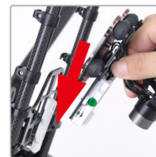
4.2 Chute to camera fixing board
