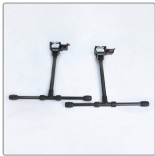
2.1 Prepare skid landing set
