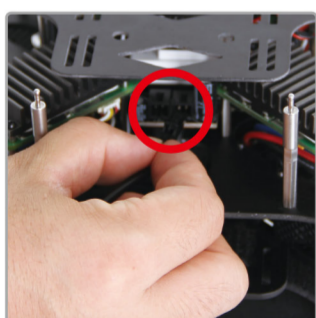
4.5 Insert the black side of power cable to port of power board
