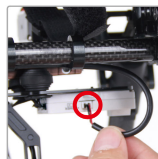
4.7 Insert the white side of power cable to port of gimbal controller
