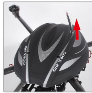
6.3 Put the GPS signal cable and support tube through the canopy and then install the canopy
