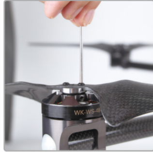
7.3 Install propeller (rotating mark must match with body)
