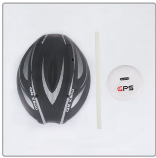
6.1 Prepare GPS module, support tube, canopy
