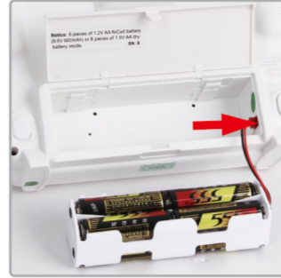
8.1 Connecting the battery
