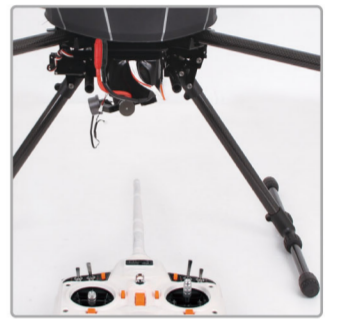
9.6 The red LED flash quickly till light out which means calibration finished. Please reconnect the aircraft power after calibration.
