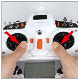
9.1 Enter compass calibration
