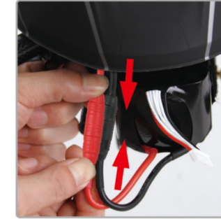
8.3 For safety, please follow the blew steps to connect/disconnect the power. Please connect the black connectors first and disconnect the red connectors when connecting the power; Please disconnect red connectors first and the black connectors later and when disconnecting the power.
