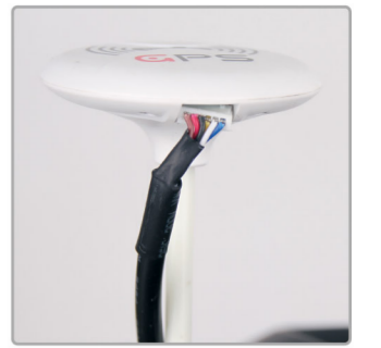
6.5 Connect the GPS signal and insert GPS module port
