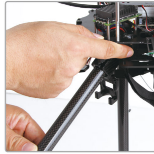
1.3 Press spread key, spread motor fixed tube parts upwards
