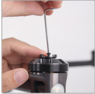
7.2 Take off the fixed crews of propeller
