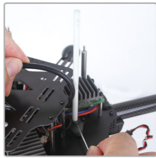
6.2 Put the support tube into the fixing block to fix.
