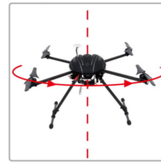
9.4 Horizon level 360° rotation (Rotate the aircraft, from 0° to 90°, 180°, 270°, 360°, all need to pause for 1 second.)
