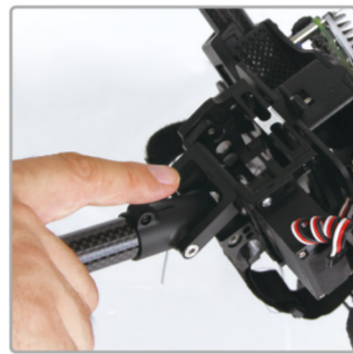
2.2 Put it into tripod sliding chute AUX3 connect to AUX3 AUX4 connect to AUX4
