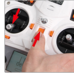
8.2 Turn the MIX/FMOD/GEAR switch to "0" position and keep the throttle at the lowest position then turn on the Radio
