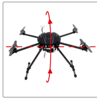
9.2 Forward & backward 360° rotation (Rotate the aircraft, from 0° to 90°, 180°, 270°, 360°, all need to pause for 1 second.)
