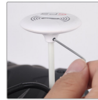
6.4 Mount the GPS module to the top of the support tube and fix it.
